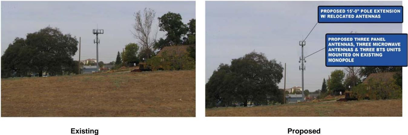
The City encourages co-locating antennas on existing towers wherever feasible; as facility and site sharing results in minimal impacts to the surrounding properties, while also providing the necessary improvements needed to enhance service capacity.
